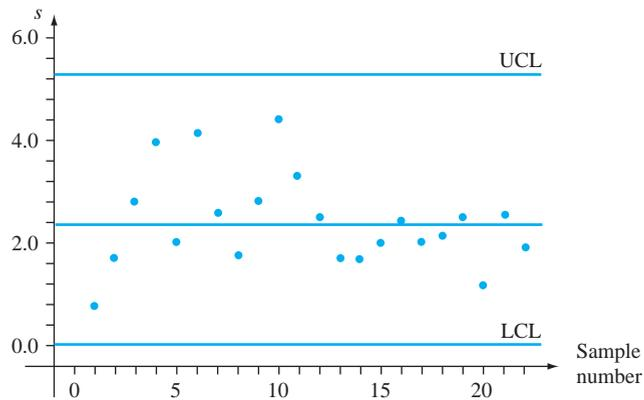
**Figure 16.3**  $S$  chart for stress-resistance data for Example 16.4
